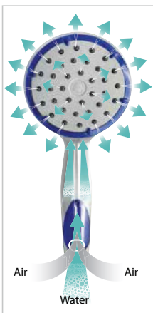
Jets of air flow into the showerhead increasing the showers power.
